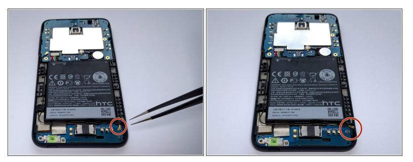
• Using Tweezers, disconnect antenna wire.
