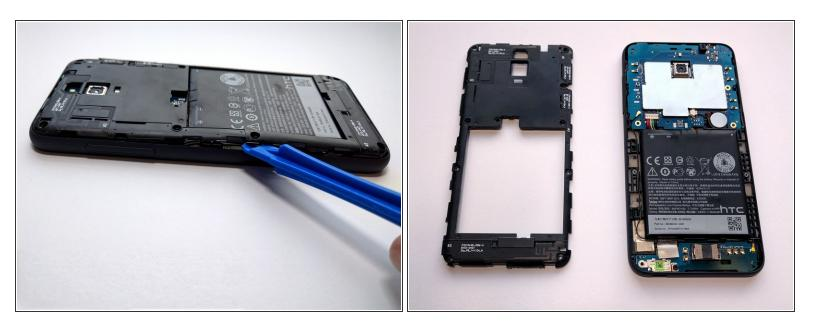
• Using plastic opening tool, remove the black plastic circuit cover.
