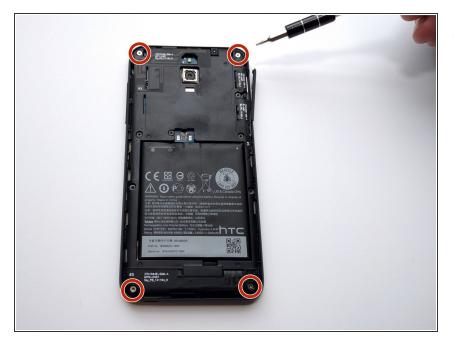
Using Torx T5 Screwdriver, remove the four 5mm silver torx head screws.
