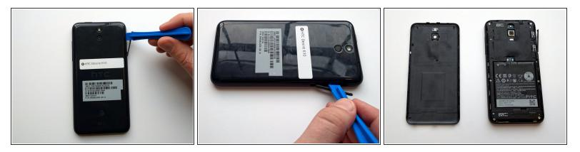
• Using plastic opening tool, take off the back cover of the phone.
