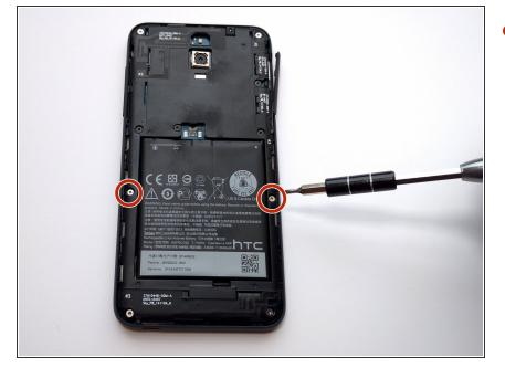
Using Phillips #000 Screwdriver, remove the two 2.5mm phillips head screws.
