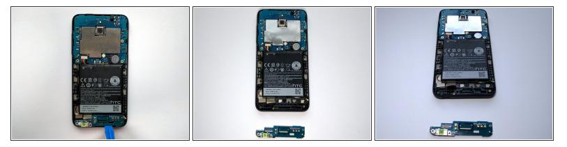
• Using plastic opening tool, pry up green plate and pull outward.
