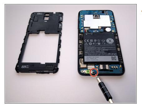
Using Torx T5 Screwdriver, remove the 4mm black torx screw.
