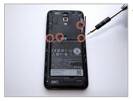
• Using Torx T5 Screwdriver, remove the four 4mm black torx screws
