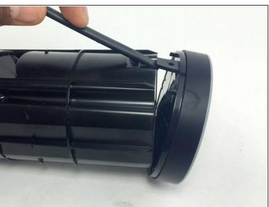
Unclip and remove the top volume ring assembly from the Echo.
