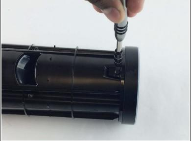
Remove the 9.7 mm T10 Torx screw from the opposite side of the Echo.
