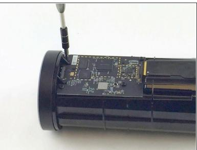
Remove the four 9.7 mm T10 screws.
