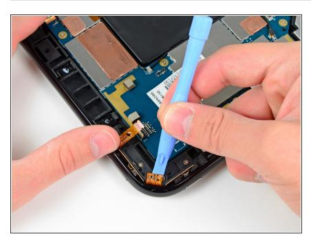
Use the edge of a plastic opening tool to peel the ambient light sensor off the body of the control button assembly, revealing a hidden screw.
