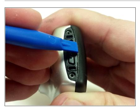
Slide the plastic opening tool into the seam between the front and back sections of the case and apply a small amount of force to pop the case open.
