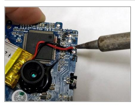
Melt the soldered battery connections with a soldering iron and gently pull the battery wires away.
