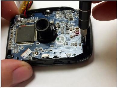
• Using a P1 screwdriver, remove the 4mm screws holding the motherboard into the case.
