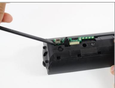
With the black spudger, carefully wedge out the I/O board.
