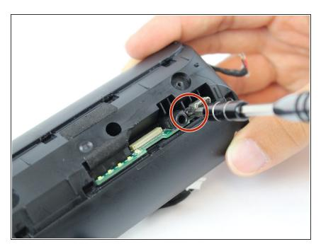
Remove the one 7.0 mm Phillips #1 screw that connects the I/O board to the casing.
