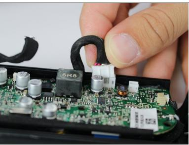
Using the black spudger, carefully remove the cord connecting the battery to the motherboard.
