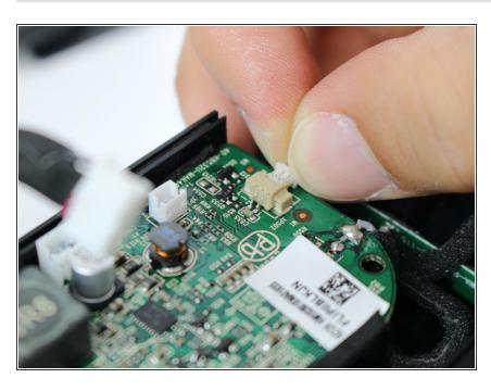
Carefully remove the cable connecting the nfc chip to the motherboard.
