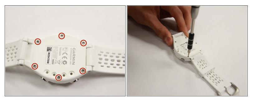
• Remove the six T5 Torx 6.32mm screws securing the back cover to the watch.
