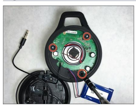
Remove the three 7mm philips head screws on the outer edges of the device.
