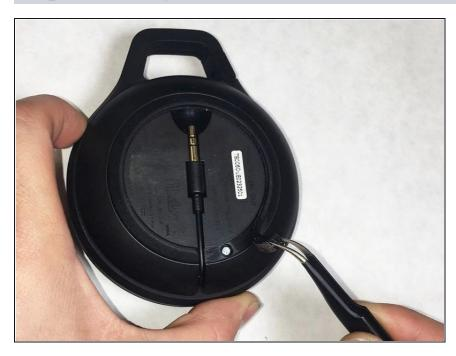
Use the angled <u>tweezers</u> to carefully pull the rubber bumper off the back side of the device
