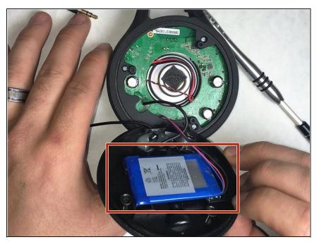
• The battery is adhered to the back cover of the JBL Clip Plus, slowly lift the battery away from the case, using a spudger to pry the battery away from the adhesive.
