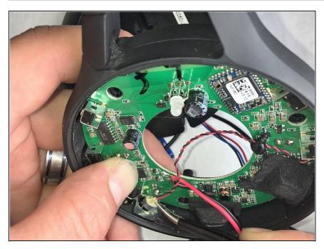
Gently push the motherboard away from the microphone, this will allow you to remove the microphone.
