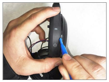
Use the plastic prying tool to gently remove the face of the speaker from the body.
