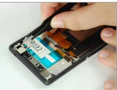
With your fingers, or nylon spudger if necessary, remove headphone jack fastening cover, casing, and sticker.
