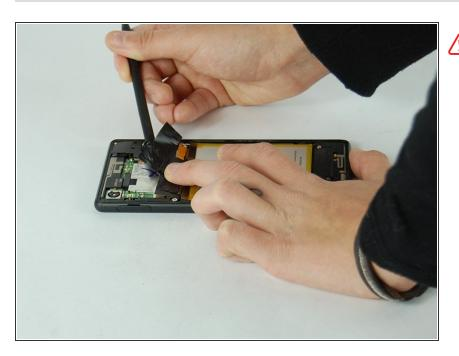
Remove copper plated tape and any other securing adhesive with a nylon spudger. Remove carefully, as it has the potential or tear if too much force is used.
