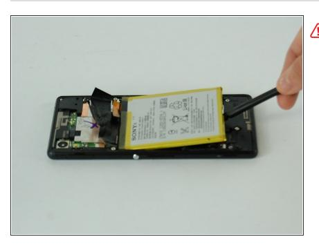
Pry the battery from the phone with the nylon spudger. There is a small amount of adhesive underneath the battery, so a bit of force is required. The battery is malleable, so it is possible to dent the battery if too much force is applied in one spot.
