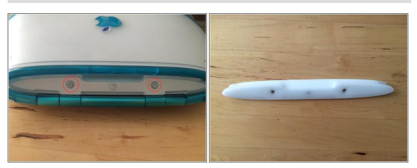
• Use a t8 Torx driver to unscrew the two screws holding in the back cover, then remove the cover.
