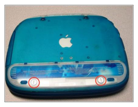
Use a coin to unscrew the battery cover, and remove battery.
