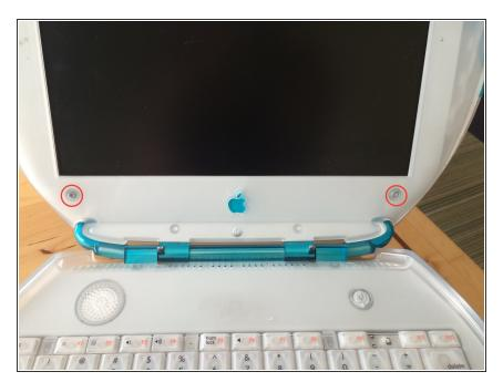
Open the screen, and remove the two t8 Torx screws holding the bezel in place.
