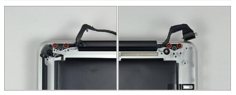
Remove the two outer T8 Torx screws securing each side of the display bracket to the upper case (4 screws total).
