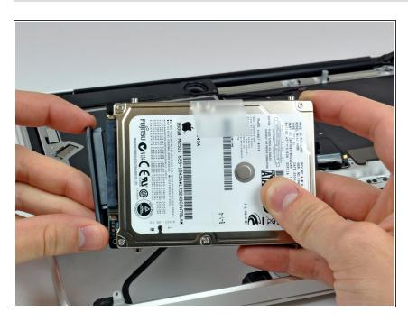
Disconnect the hard drive by pulling the hard drive cable connector away from the drive.
