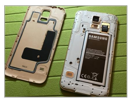
Use your fingernail or a pry tool to remove the rear plastic cover of the device, by pulling back on the edges.
