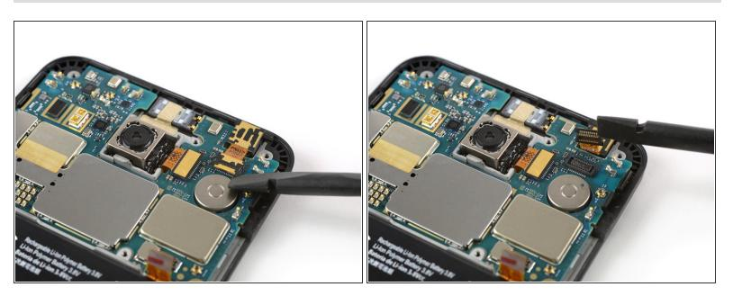
Use the flat end of a spudger to pry up and disconnect the front-facing camera flex cable.
