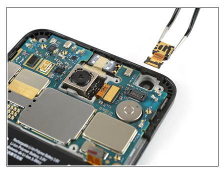
Use a pair of tweezers to remove the front-facing camera from its recess. If possible, turn on your phone and test your repair before installing new adhesive and resealing the phone.
