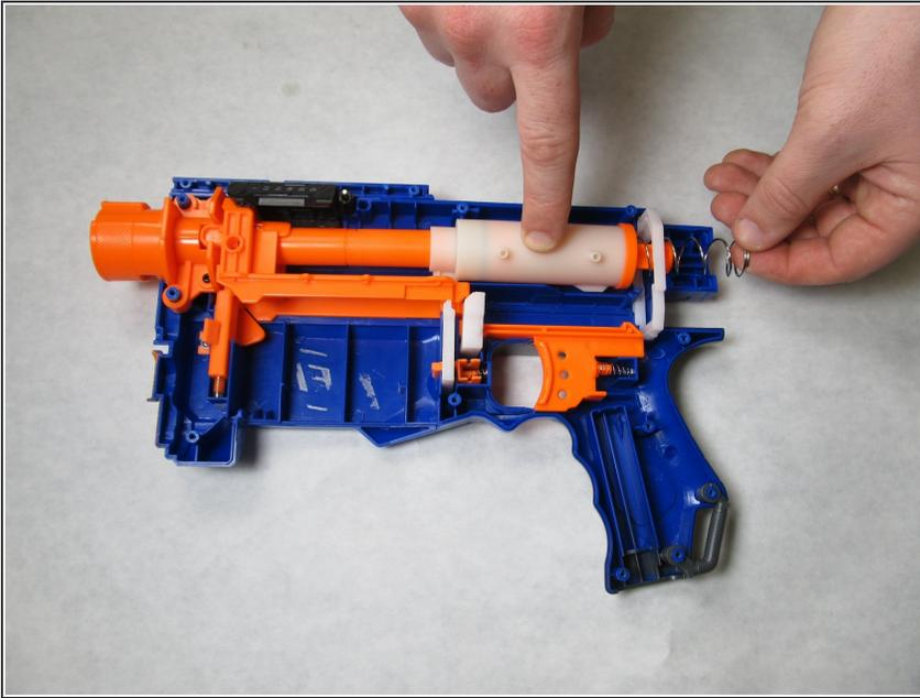
**⚠** The firing spring may be energized. If so, carefully release and spring pressure before proceeding.
