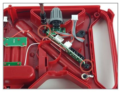
Remove the two Philips #1 screws that secure the I/O board to the case.
