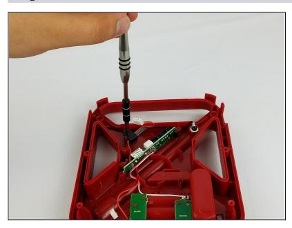
• Just above the I/O board, there is a small clip securing the wire to the motherboard. Remove the Philips #1 screw and lift it up.
