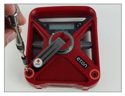
On the bottom of the device case's face are two T10 screws.
