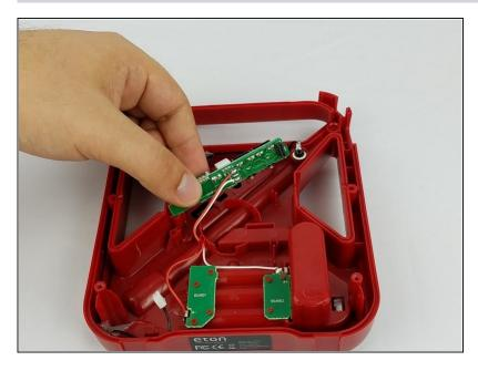
Gently lift the I/O board straight upwards to remove it.
