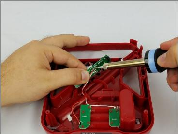
• Unsolder the red and white wires where the backup batteries connect to the I/O board.
