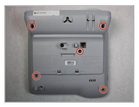
Remove the five 4mm X 10mm screws from the back cover of the device using a Phillips #1 screwdriver.
