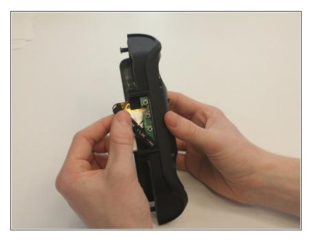
• Remove the rubber covering from the buttons.
