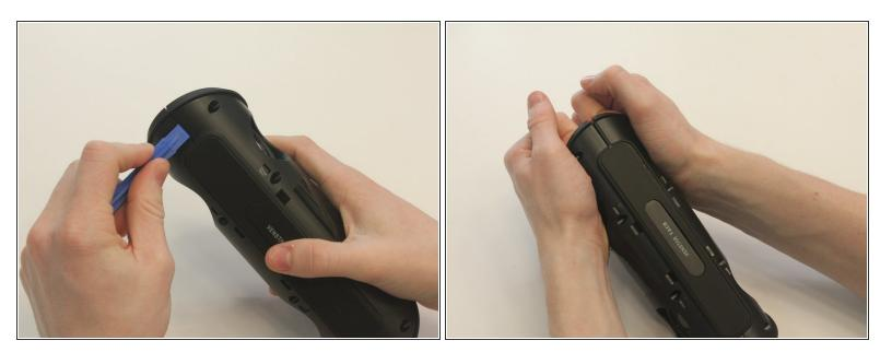
From the same side you just unscrewed, use a plastic opening tool to unwedge the inner cover on both sides of the base.
