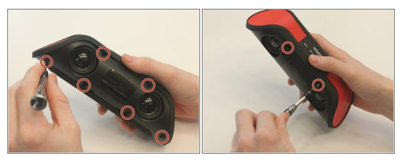
Using a <u>Phillips PH0 3 mm-bit screwdriver</u>, remove the six screws on the inner layer of the Taco.
