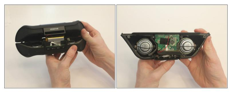
• Slide off the inner cover. It pulls apart and is held on by a small amount of glue.
