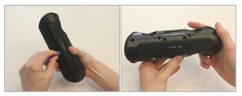
• Repeat the previous step on the opposite side to remove the other outer casing.
