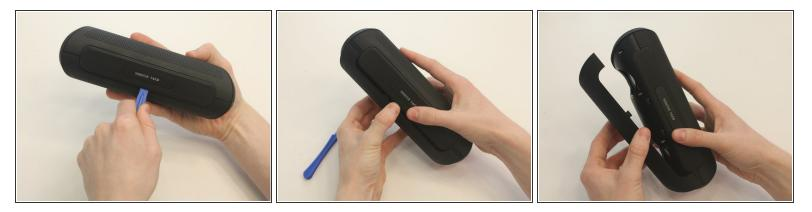
Starting with the Taco on its side, use the plastic opening tool to pop off the outer casing near the base.
