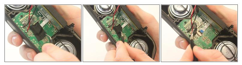
• Remove the black fabric covering the logic board.
