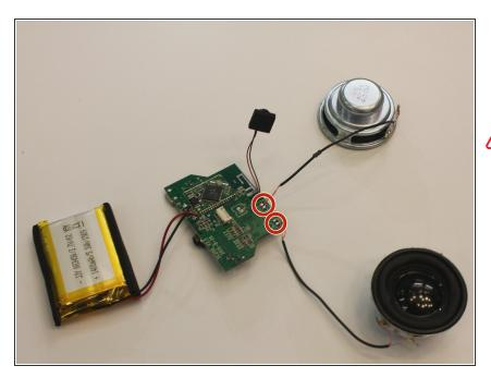
Using a portable soldering iron, melt the solder on the black speaker wires on the logic board.
