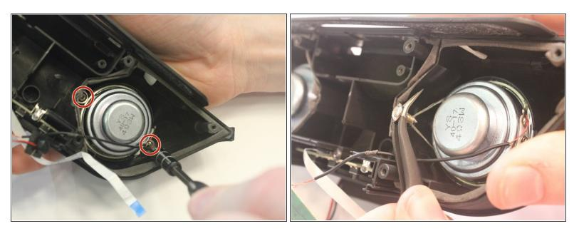
• Using the Ph1 screwdriver, unscrew both of the 2.5mm screws on either side of the speakers.
