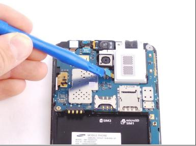
Unhook the ribbon cable clip with the plastic opening tool and remove the audio jack.
