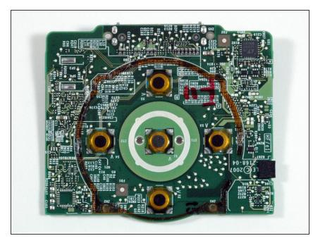
• A (prettier) view of the bottom of the logic board.
