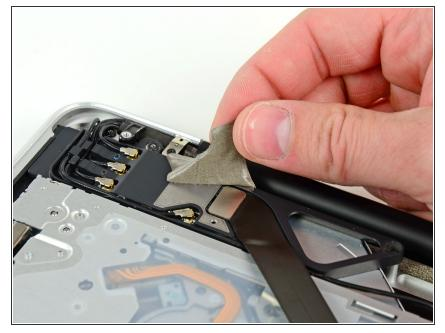
• Peel back the piece of EMI tape covering the AirPort/Bluetooth cable on the AirPort/Bluetooth housing.
