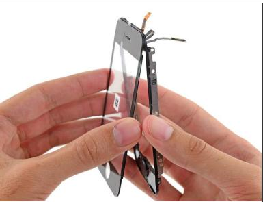
Ensuring that the upper cables are folded clear, align the top of the front glass with the front panel frame.
