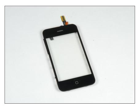
This is what should be left after removing the LCD.
