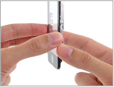
Press the front panel and front panel frame together, ensuring the the home button ends are aligned.
