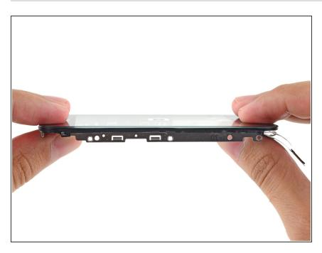
Firmly press both ends of the phone to ensure the attachment of the adhesive.
