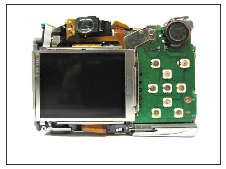
Once the ribbon connecting the back cover is removed, the back of the camera body should look like this.
