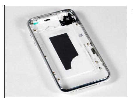
• The rear case and attached front bezel remain.
