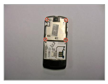
Remove the four (4) T6 Torx screws from the back of the metal back plate.
