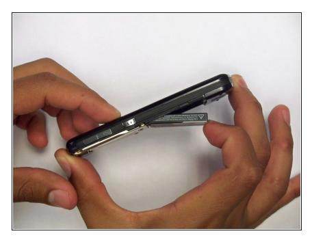
Remove the battery on the back of the Motorola phone by pulling it away from the back of the phone.
