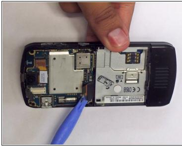
Carefully separate the two connectors from their sockets on the motherboard using the flat end
