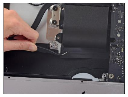
• Peel off the tape covering the exhaust duct.
