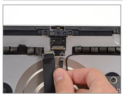
Disconnect the microphone connector from its socket on the camera board.
