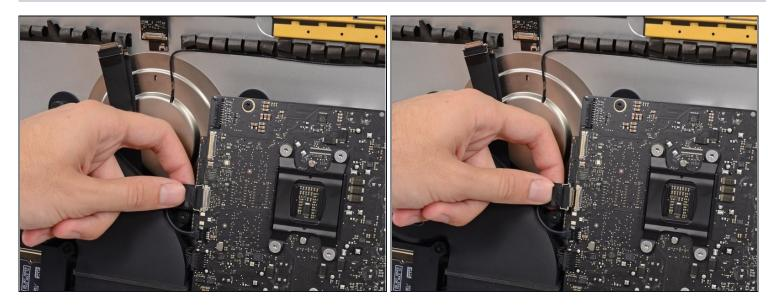
• Pull the camera cable straight away from its connector on the logic board.
