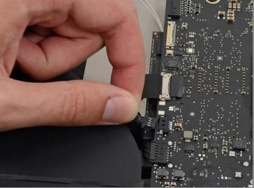
Gently pull the fan cable connector straight away from its socket on the logic board.
