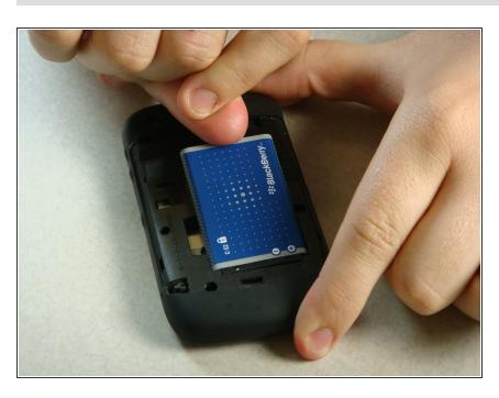
Remove the battery by pulling up from the top of the battery.
