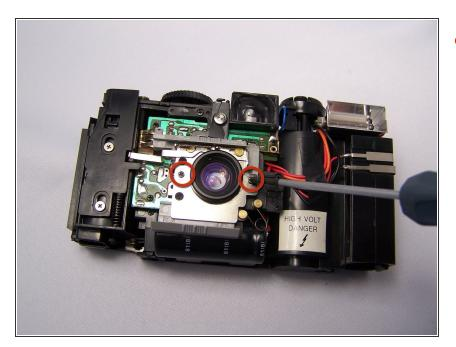
Remove the two 6.2mm Phillips screws on either side of the lens securing the metal plate.
