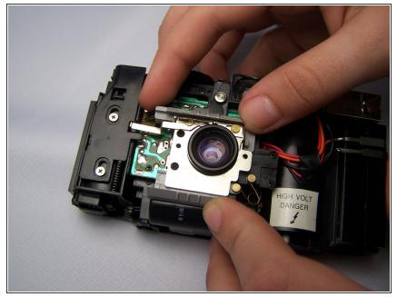
Pull aside the plastic piece resting atop the metal lens plate in order to access the other screws.
