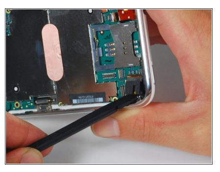
Use a spudger to gently remove the camera retaining clip, (formerly secured by the removed screw) and gently pry the camera up and out of its housing in the rear panel. The camera cannot be removed entirely yet because it's connected to the bottom of the logic board.
