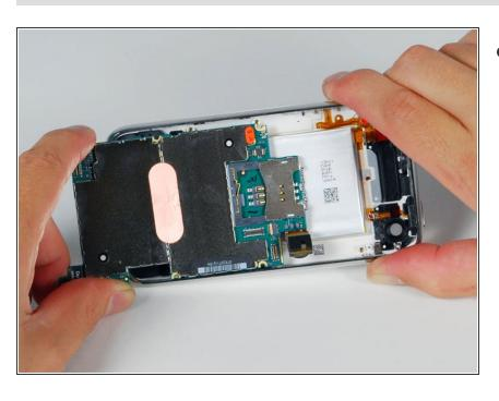
Slide the logic board towards the dock connector and out of the iPhone.
