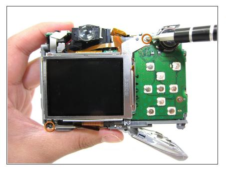
Use a #00 phillips head screwdriver to remove 2 3.34mm phillips screws holding the LCD screen in place.
