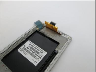
Gently use the plastic opening tool to set the tab free. This tab is used to hold the screen in place.
