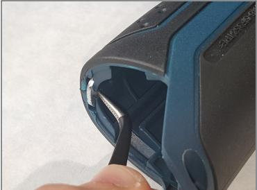
• Locate the clip that connects the two halves of the outer casing on the rear edge of the battery shaft. \*Use the angled <u>tweezers</u> to remove the clip.
