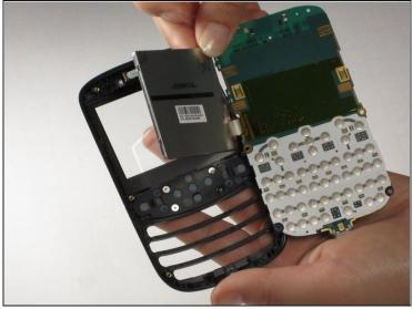
• Using a spudger, remove the display screen from its cell within the front case. Insert the spudger next to the LCD on the opposite side of where the motherboard is attached.
