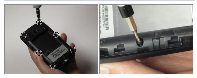
• To remove the case, use a small, pentagonal screwdriver to unscrew the 6 screws that can be found around the edges.
