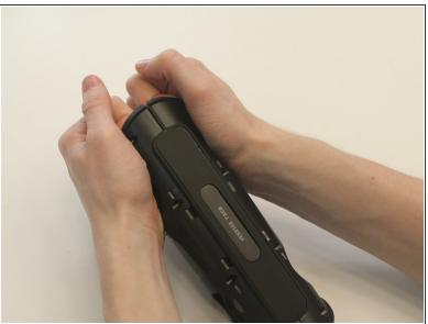
From the same side you just unscrewed, use a plastic opening tool to unwedge the inner cover on both sides of the base.
