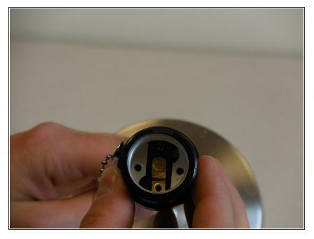
• Set the sliver threaded socket into place. Turn the socket to align the two screw holes.
