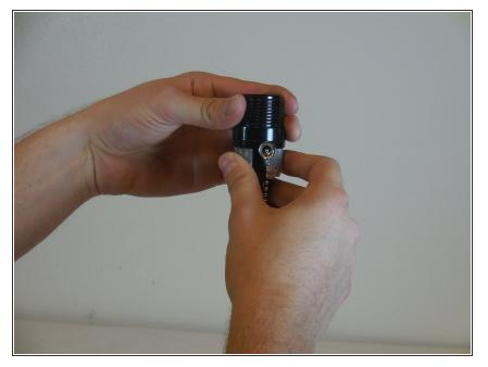
• Unscrew and remove the outer black socket body.
