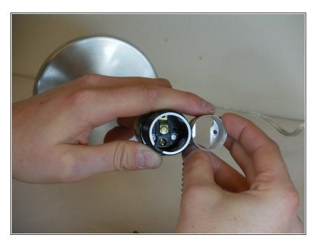
• When the screws are removed, the threaded socket will pull out.
