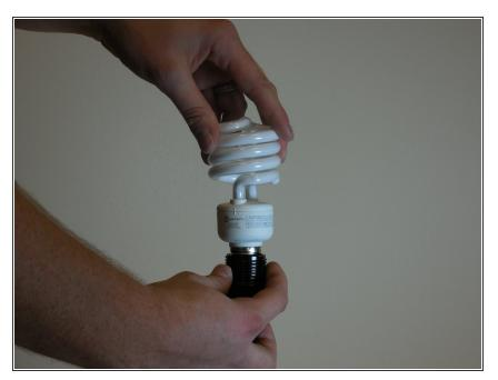
• Unscrew the light bulb from the socket then remove the lamp shade.
