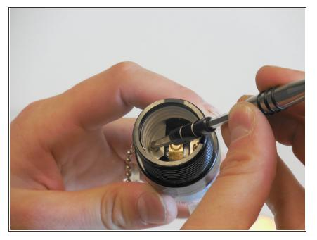
Remove the two screws from the bottom inside the socket. These screws hold the silver threaded socket in place.
