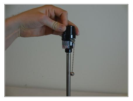
Pushing downward to hold the socket in place, screw the black outer socket back in place to secure the switch.
