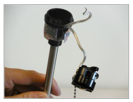
Pull the socket base/switch assembly out of the base to gain access to the screw terminals on the sides.
