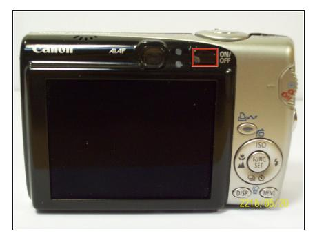
Turn off the camera by pressing the power button above the LCD screen.
