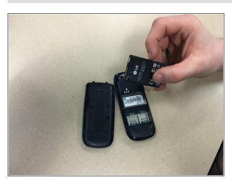
Gently remove the battery from the device.
