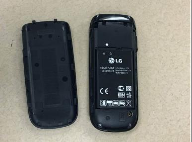
Slide the back down towards you and remove the back cover. You should hear a slight click as the cover comes off.
