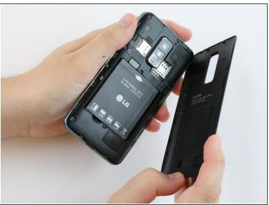
Using your thumbnail, lift up on the notch in the middle of the bottom side of the phone.
