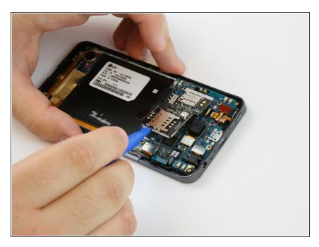
Hook the plastic opening tool underneath the plate and gently lift it up.
