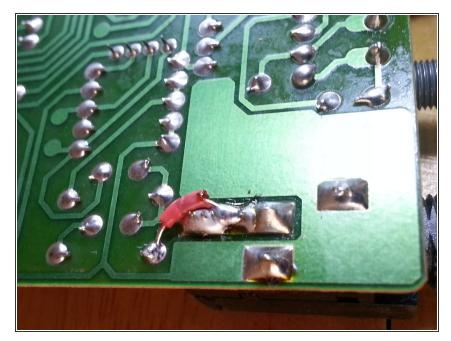
I soldered a bridge between these two tabs that share a connection and across the part of the trace I shaved. I also added a jumper to back up that trace.
