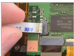
• Use two fingers to remove the two ribbon cables in the bottom left corner of the motherboard.
