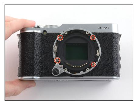
Remove the four 4.3 mm screws securing the sensor to the front case.
