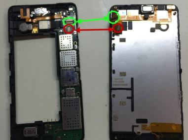
disconnect the two connectors here: Green, and Red.
