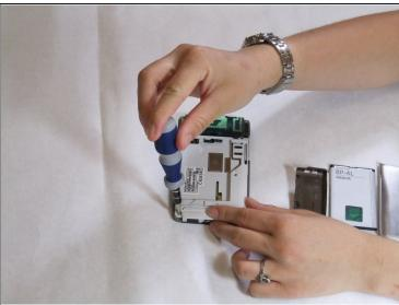
Remove the four screws that secure the front cover to the rest of the phone using a T7 screwdriver.
