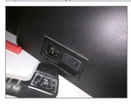
⚠ First, start by putting appliance into standby mode. Then put general switch to 0. Finally, disconnect power cord.
