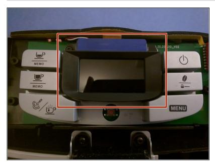
Remove the LCD black plastic frame. It is simply placed into two necks.
