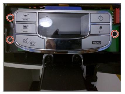
Remove the three screws of the touch panel frame.
