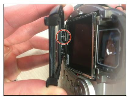
As you start to reassemble, note the grey extension at the bottom of the black screen cover. Apply pressure to the bottom of the cover and slide upwards onto screen.
