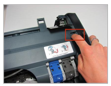
Depress the plastic tabs marked in red to release the cover from the sides.
