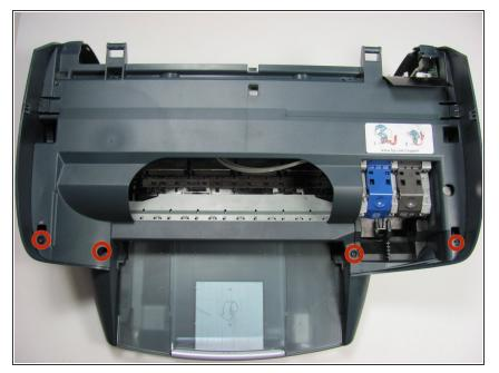
Remove printer carriage cover by unscrewing four black coarse thread T-10 torx screws marked with red circles.
