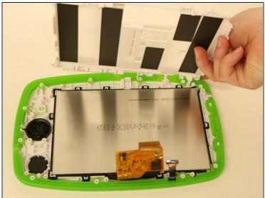
• Carefully lift out the plastic plate and set it aside.
