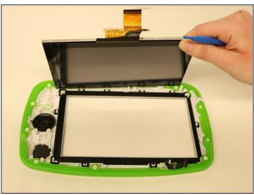
• The screen is now completely accessible and can be lifted out of its cradle. Use the plastic spudger to safely and carefully lift the screen up.
