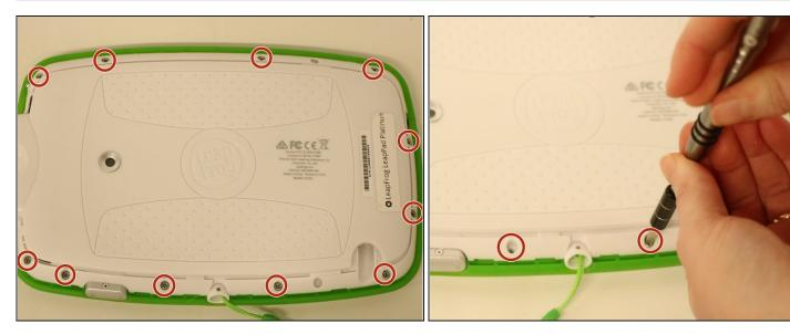
• Remove the 11 Phillips screws (8.0 mm) located around the edge of the back cover with a Phillips screwdriver.
