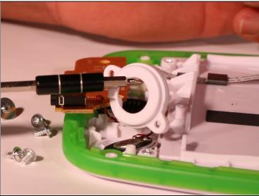
• Locate the circular plastic speaker cover, remove the two 5.0mm Phillips screws holding it in place, and gently lift the cover away from the device.
