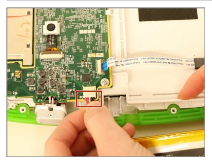
The battery has red, black, and white wires that are all connected to the motherboard through a plastic clip. Unplug this plastic clip to fully remove the battery from your device.
