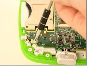
• Remove the three 4.0 mm Phillips screws located in the corners of the motherboard.
