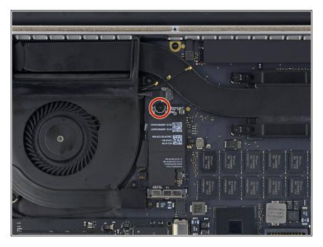
Remove the single 2.9 mm T5 Torx screw securing the AirPort board.
