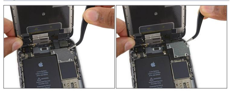
• Remove the display cable bracket.
