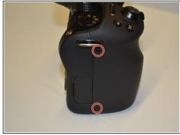
Unscrew the nine 4mm Phillips head screws surrounding the body of the camera. They are located on the bottom of the camera and both sides of the camera.
