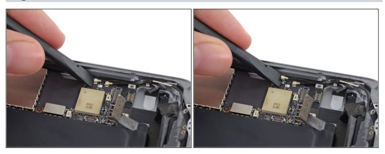
• Use the flat end of the spudger to pry the antenna connector up from its socket on the logic board.
