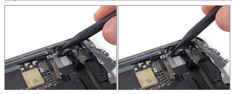
• Use the tip of a spudger to pry the small metal retaining clip off the antenna cable.
